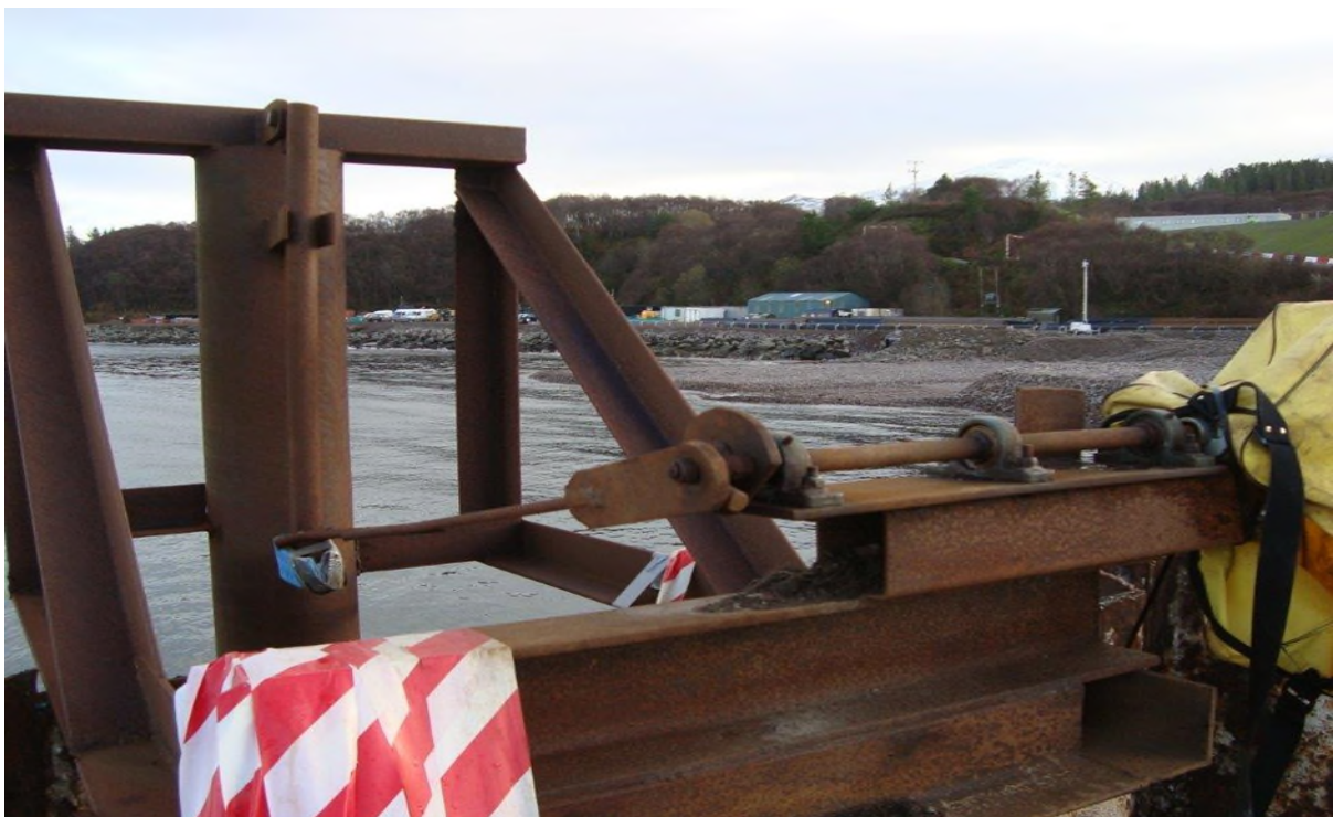
Figure 7.6.1 A noise generator similar to the one proposed to be used at the Stornoway DWP development to implement soft start procedures
