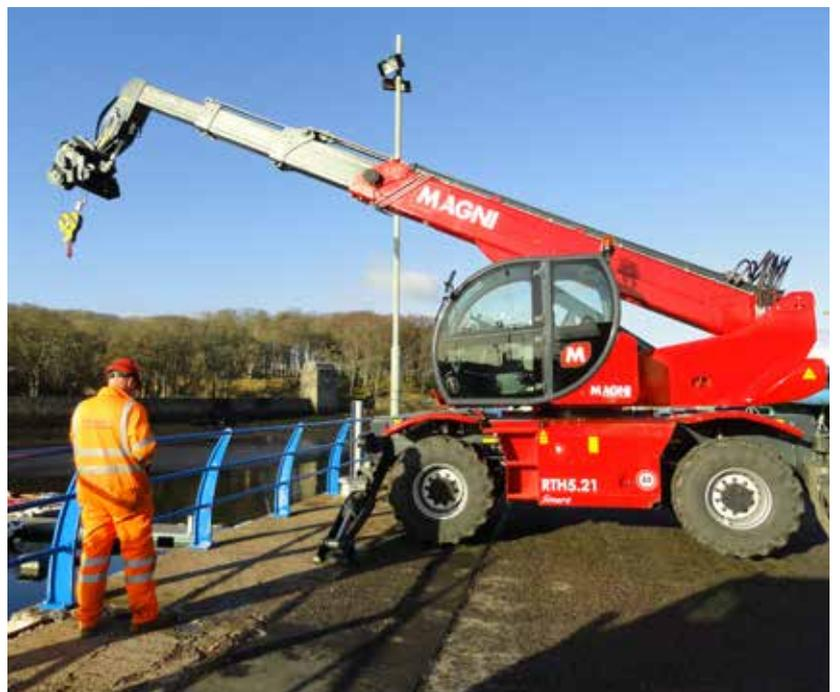
The telehandler pictured above is lifting engine out of leisure vessel "Blue Star"
